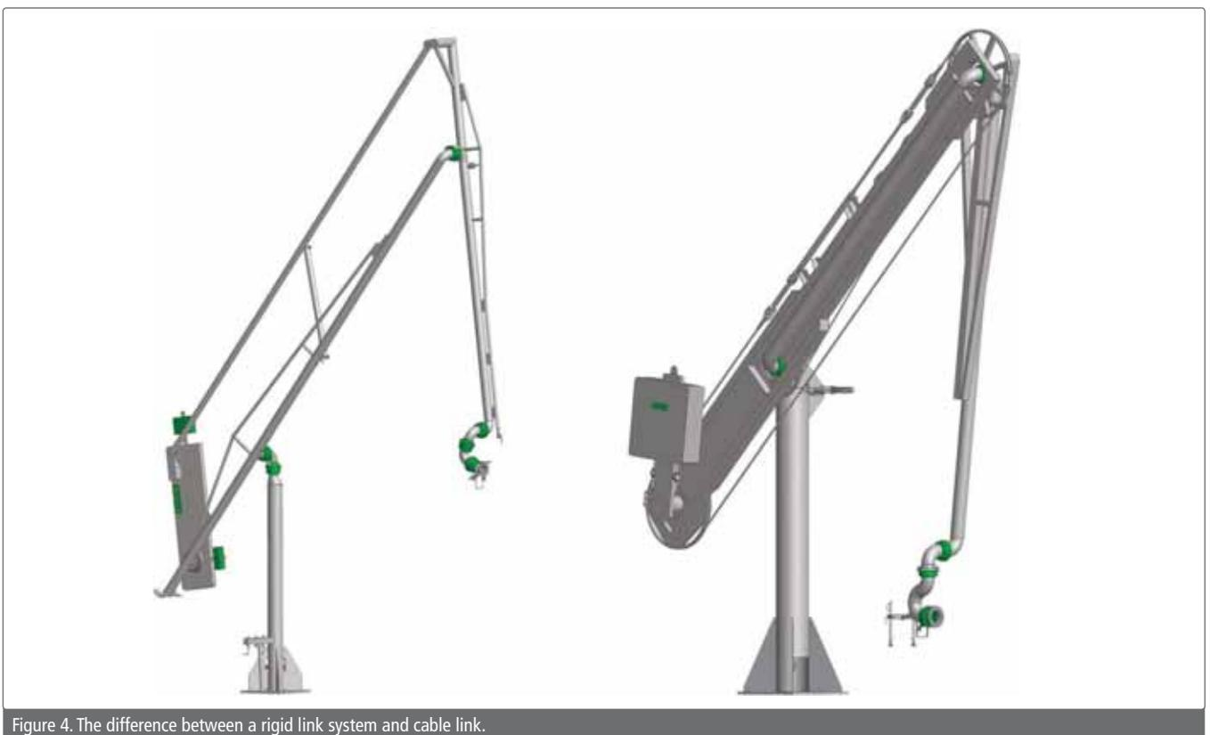
To increase job satisfaction and job performance, the facility and the operation of loading arms and maintenance should be designed through the eyes of operators and maintenance crew and suited for one man operation. For example, flexible wires with pendants for regular loading arm control should be avoided, as they can cause accidents and are prone to getting damaged, thus causing unexpected movements of the arms.
