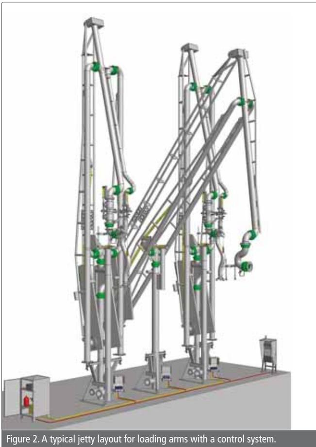
Connections made by marine loading arms achieve a fully rigid connection, still with the possibility to follow all the ship's movements by the use of swivel joints in between the steel pipes, and so solve the disadvantages of loading hoses. They can also be executed with automatic 'no spillage' emergency release couplers
